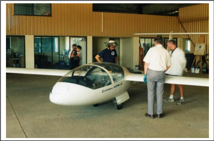
One of the Caproni Califs. This is an all-metal aircraft with side by side seating
