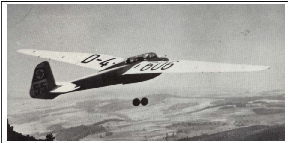
The Kranich 2-seater. A high performance machine when it was introduced in the 1930s. This version, with the jettisonable wheels had a best glide ratio of 24:1. The ones flown by Dennis at Lubeck had the undercarriage fixed in place.
